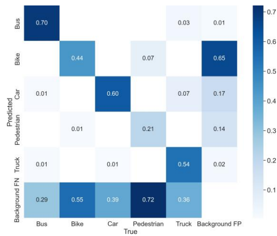
Figure 6. Normalized Confusion Matrix of YOLOR-P6 model on the input size 1280 × 1280.
